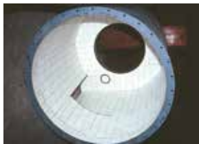
Cycloonbekleding met Kalocer in 6 mm dik
